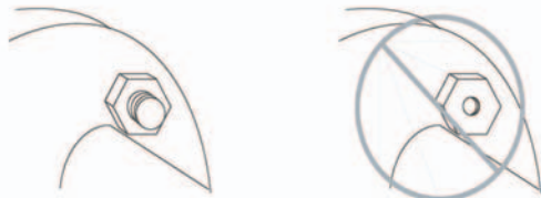
Fig. 4. Basic proper bolt length.
